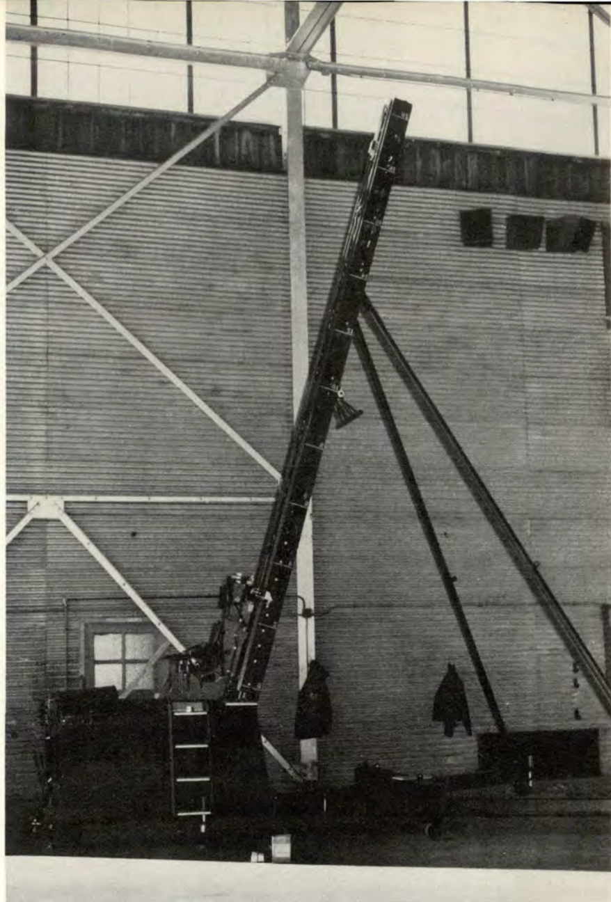
The trainer accomplishes two things: It enables a student to review procedures and to feel the actual physical sensation of an ejection.
